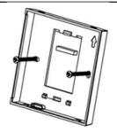
4. Put the connected thermostat onto the back panel in the wall, then fix it with the two screws in the packing box.
